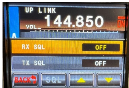
Figure 12 Here is where the repeater may be told that it is to use sub-audio tones. The frequencies of the tones themselves may or may not have been already set. Those are separate functions.
