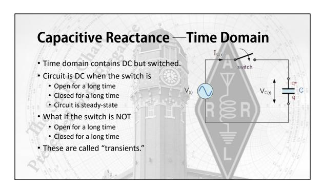
Think of the time domain as controlled DC. It is DC in "steady-state" when all transients have settled. The circuit is NOT in steady-state when the switch has NOT been open or closed for "a long time." We call these transients.
