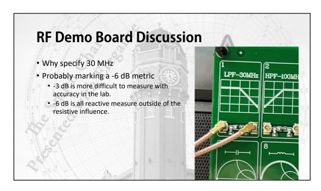
So, now let us entertain the discussion of why 30 MHz. No doubt this is to more precisely locate the roll-off point. At -3 dB the resistance and reactance are equal. But at -6 dB the reactance far outweighs the resistance making its measurement more predictable.
