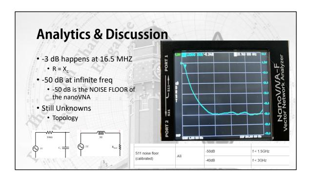
We already noted -3 dB at 16.5 MHz where the resistance equals the reactance. But we also are seeing a maximum gain at about 100 MHz. This is instrumentation error. The nanoVNA is only able to measure a noise floor as low as -50 dB. Know your laboratory instrumentation limitations. But what is still unknown is the topology of the actual circuit of the RF Demo Board. It could be inductive or it could be capacitive. Let us switch to a Smith Chart view in the next slide.
