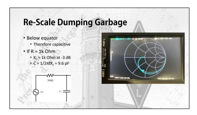
The smith chart shows that the circuit only contains capacitance since there is no trace in the Northern hemisphere. We are showing a quantified capacitance in this slide but we could have done that in the previous slide.
