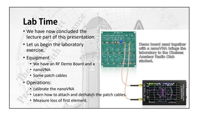
Let us begin the laboratory exercise. You have a nanoVNA, patch cables, and the RD Demo Board. On our list of operations we are going to first calibrate the nanoVNA, then learn how to safely attach and detatch those fragile patch cables, and finally we will measure the first element of the RF Demo Board—its low pass filter.
