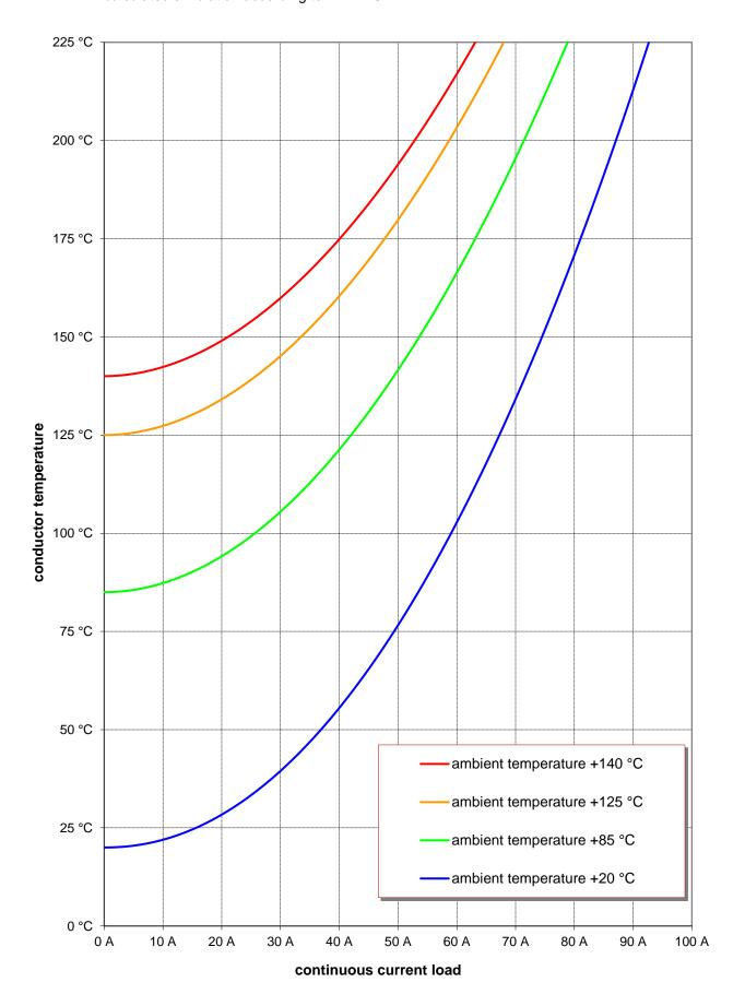
Annex: Short-term current loading on conductor as a function of ambient temperature calculated simulation according to LV112-3
