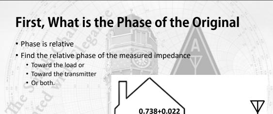
The first order of business is to find the phase of the original configuration. Cable type and length are irrelevant because we already know the vector impedance at the original feed-point entrance. We could have done this before moving the ham shack but at that time there was no need for this information.
