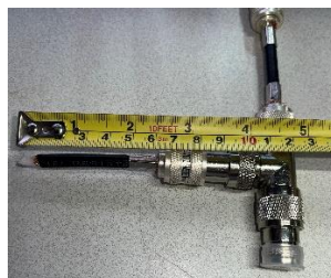
Figure 11 Shown here is the effective length of the open-end stub itself.
