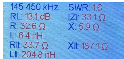
Figure 1 The vector impedance measured looking into the transmitter feed line is shown as 32.6 + j5.90 Ohms
