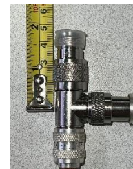
Figure 12 It might be easily missed, but there are 4mm of length added to the antenna feedline coming into the stub.
